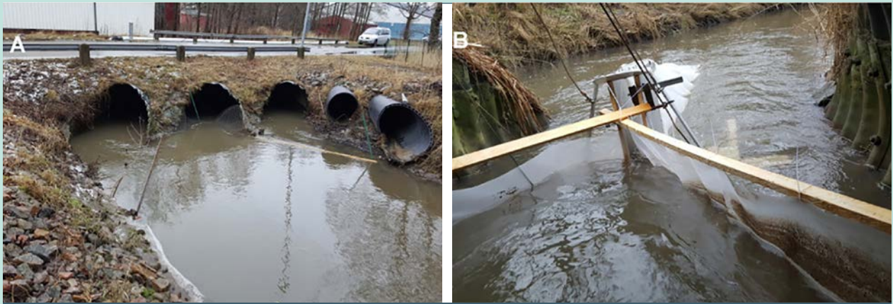
Figure 10: (A) and (B) 300 µm mesh nets collecting nurdles in the Orust-Tjörn Fjord system, Stenungsund, Sweden chemical cluster. February 2016. lix
